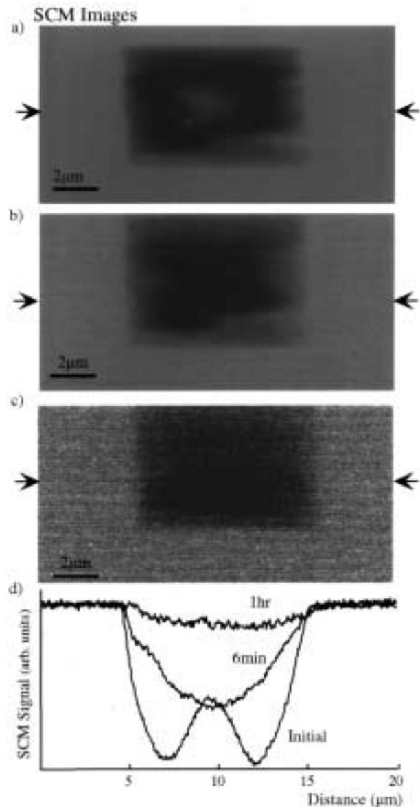
FIG. 2. SCM images obtained at 0 V dc sample bias of a locally charged region of the doped  $\text{Al}_x\text{Ga}_{1-x}\text{N}/\text{GaN}$  HFET epitaxial layer structure and surrounding uncharged regions, obtained (a) immediately, (b) 6 min, and (c) 1 h after charging. (d) Line scans extracted from the images (a)–(c) at the locations indicated by arrows.
