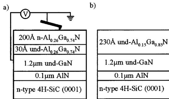
FIG. 1. Schematic diagrams of (a) doped and (b) undoped  $\text{Al}_x\text{Ga}_{1-x}\text{N}/\text{GaN}$  HFET epitaxial layer structures. Sample and probe tip geometry and electrical connections are indicated schematically in (a).
