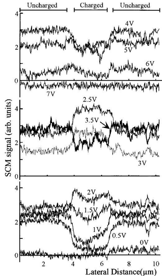
FIG. 3. SCM line scans across a 10  $\mu\text{m} \times 2.5 \mu\text{m}$  sample region charged at 9 V sample bias, obtained at imaging bias voltages ranging from 0 to 7 V. Bias voltages employed during SCM imaging as well as charged and uncharged regions for all line scans are indicated.
