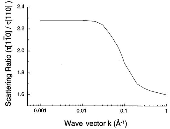
FIG. 6. Calculated ratio of interface roughness scattering times as a function of  $k$  using the interface roughness parameters determined by STM for the 17-Å InAs/50-Å Ga<sub>0.75</sub>In<sub>0.25</sub>Sb superlattice. The scattering time ratios should be directly proportional to the carrier mobility ratios in the superlattice. The anisotropy in the calculated scattering times is in semiquantitative agreement with the measured anisotropy in Hall mobility in the superlattice.
