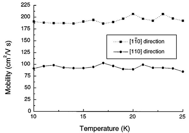
FIG. 5. Measured Hall mobilities for the superlattice as functions of temperature and direction. The mobility is observed to be larger in the [1 $\bar{1}$ 0] direction than in the [110] direction of the superlattice.
