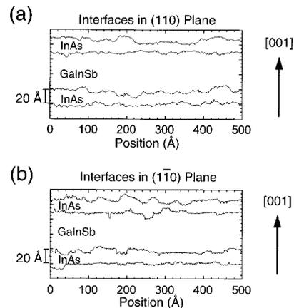
FIG. 2. Representative interface profiles obtained from (a) (110) and (b) (1 $\bar{1}$ 0) cross-sectional STM images of the  $50\text{-\AA}$  Ga<sub>0.75</sub>In<sub>0.25</sub>Sb/ $17\text{-\AA}$  InAs superlattice sample. The [001] growth direction is indicated.
