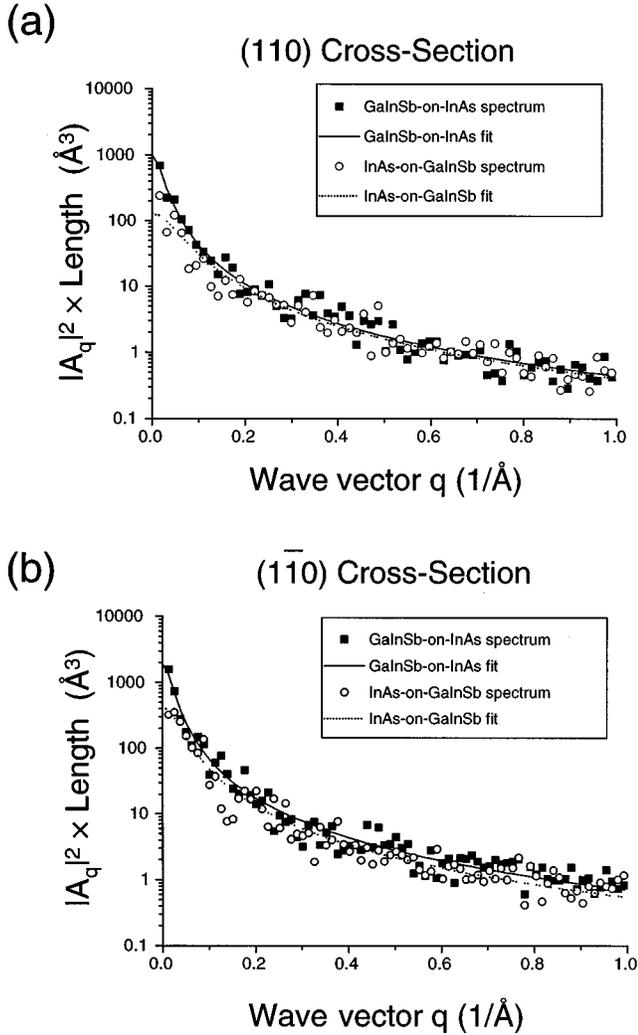
FIG. 3. Interface roughness power spectra (symbols) and Lorentzian fits to the spectra (lines) for  $\text{Ga}_{0.75}\text{In}_{0.25}\text{Sb}$ -on-InAs and InAs-on- $\text{Ga}_{0.75}\text{In}_{0.25}\text{Sb}$  interfaces from (a) (110) and (b)  $(1\bar{1}0)$  cross sections of the superlattice. Roughness amplitudes and correlation lengths for each interface type are listed in Table I.
