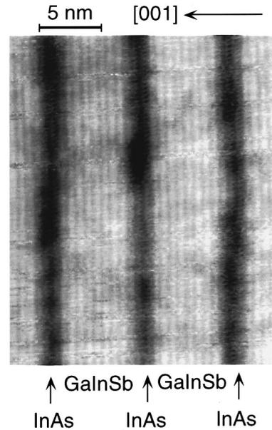
FIG. 1. High-resolution constant-current STM image of a  $50\text{-\AA}$  Ga<sub>0.75</sub>In<sub>0.25</sub>Sb/ $17\text{-\AA}$  InAs superlattice, obtained at a sample bias of  $-1.5$  V and a tunneling current of  $0.1$  nA. The gray-scale range of the image is  $2.5 \text{ \AA}$ . Monolayer roughness is visible at the interfaces between the InAs layers and Ga<sub>0.75</sub>In<sub>0.25</sub>Sb layers.
