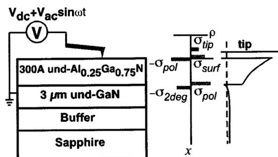
FIG. 1. (a) Schematic diagram of nominally undoped  $\text{Al}_{0.25}\text{Ga}_{0.75}\text{N}/\text{GaN}$  HFET showing geometry and electrical connections for SCM measurement. (b) Schematic of polarization-induced and free-carrier charge distribution. (c) Conduction-band diagram of tip/sample structure.
