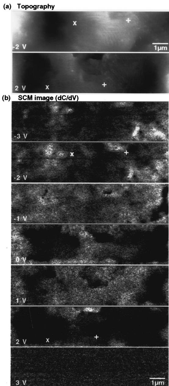
FIG. 3. (a) AFM topographic images and (b) simultaneously obtained SCM images of the  $\text{Al}_{0.25}\text{Ga}_{0.75}\text{N}/\text{GaN}$  HFET structure. The sample-to-tip dc bias voltage is indicated for each image, and corresponding locations in the images obtained at +2 and -2 V are indicated by symbols.
