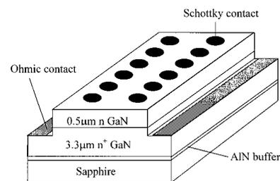
FIG. 1. Schematic diagram of Schottky diode structure fabricated from GaN grown on sapphire. The  $n^+$ -GaN layer is necessary to reduce series resistance, an essential consideration for accurate DLTS measurements.
