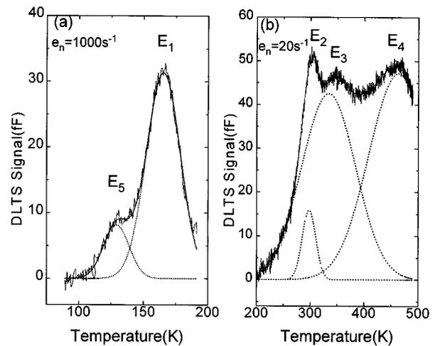
FIG. 3. (a) DLTS spectrum measured with an emission rate window of  $1000 \text{ s}^{-1}$ , a bias voltage of  $-2 \text{ V}$ , fill pulse voltage of  $+2.0 \text{ V}$ , and pulse width of 10 ms. (b) DLTS spectrum measured with an emission rate window of  $20 \text{ s}^{-1}$ , a bias voltage of  $-2 \text{ V}$ , fill pulse voltage of  $+1.5 \text{ V}$ , and pulse width of 10 ms.
